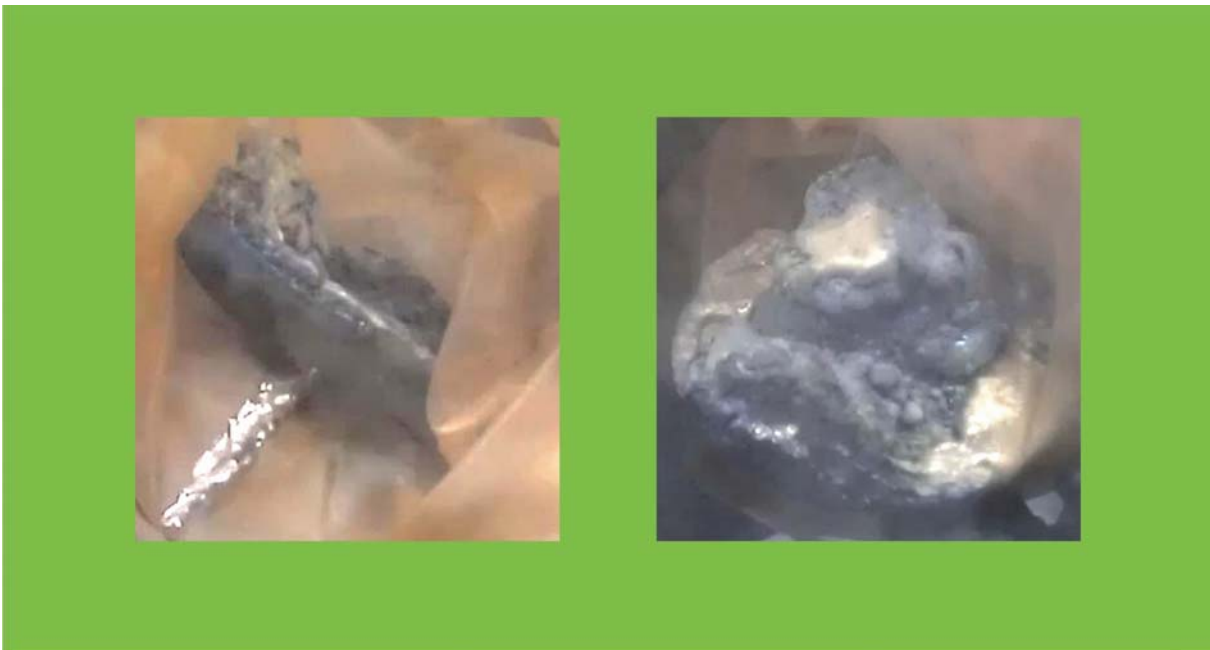
Figure 3.30. Filtrate (of the regenerated zinc alloy) to be reused in the process of cladding removal
