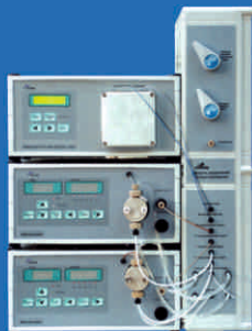
Ion chromatograph to control anion impurities
